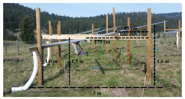
Figure 2.3. Rain-out shelter dimensions and construction blueprint
