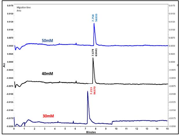
of 6.3. Thus, 40 mM imidazole solution was selected as optimized buffer concentration for the analysis. The electropherograms are shown in Figure 4.4.
