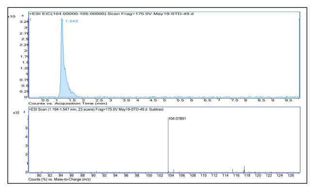
Figure C.4 - Extracted ion chromatogram and mass spectrum for choline ion present in sample 11245
