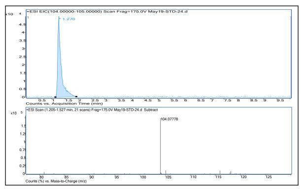
Figure C 6 - - Extracted ion chromatogram and mass spectrum for choline ion present in sample 11412
