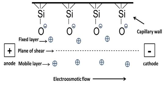
Figure 2.1 - Representation of electroosmotic flow in the capillary [4]
