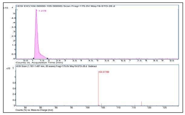
Figure C.7 - Extracted ion chromatogram and mass spectrum for choline ion present in sample 11413
