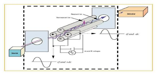
Figure 2.10 - Schematic of Quadrupole mass analyzer [64]
