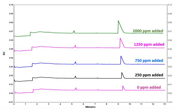
Figure B.4 - Electropherogram of sample 11245 by standard addition; choline chloride spikes added (0 ppm, 250 ppm, 750 ppm, 1250 ppm, 2000 ppm)
