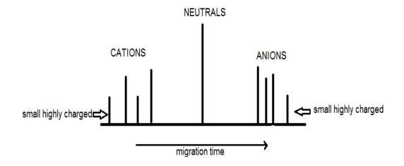
Figure 2.2 - Elution order in a capillary zone electrophoresis [51]
