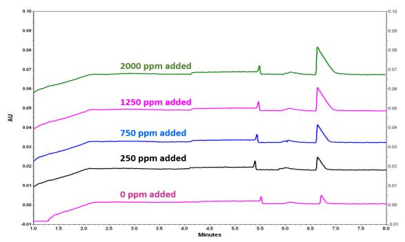
Figure B.5 - Electropherogram of sample 11411 by standard addition; choline chloride spikes added (0 ppm, 250 ppm, 750 ppm, 1250 ppm, 2000 ppm)
