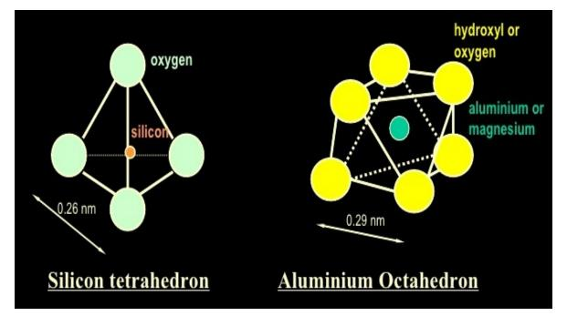
Figure 1.6 - Tetrahedral and octahedral structures of clay [13]
