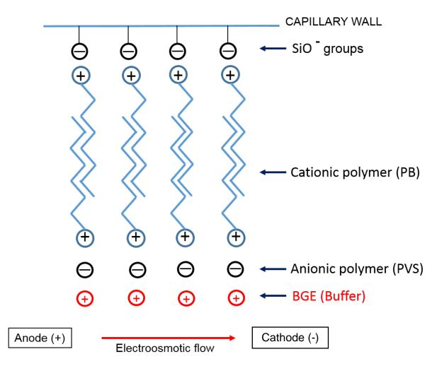
Figure 3.2 - The capillary with bilayer coating of PB/PVS [51]
