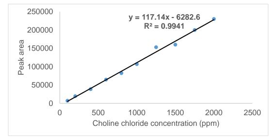
Figure 4.12 - Calibration curve of peak area of choline ion versus choline chloride concentration
