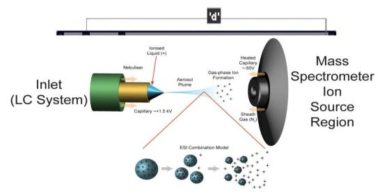
Figure 2.8 - Electrospray ionization (ESI) and ion source [61]
