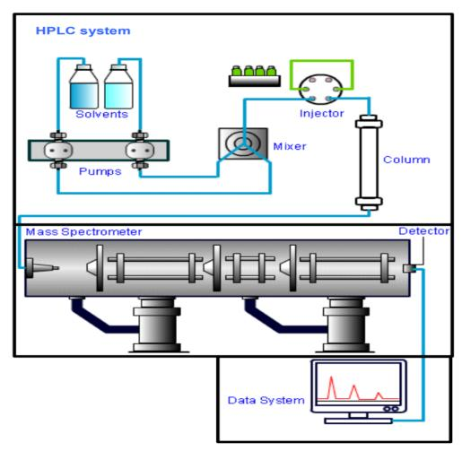
Figure 2.6 - A schematic diagram of LC/MS [10]
