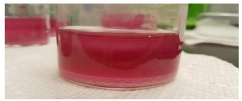
Figure 3.5 - Formed choline reinecke precipitates in the mixture
