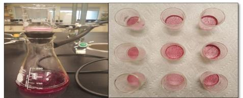
Figure 3.6 - Vacuum filtration and collected choline reinecke precipitates
