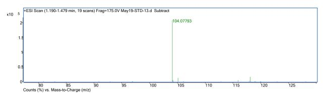
Figure 4.19 - Mass spectrum for choline present in 750 ppm choline chloride standard solution (y-axis is signal intensity and x-axis is m/z)
