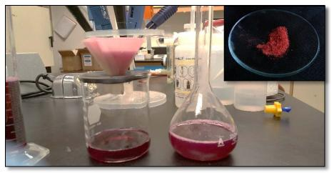
Figure 3.4 - The saturated ammonium Reinecke salt solution
