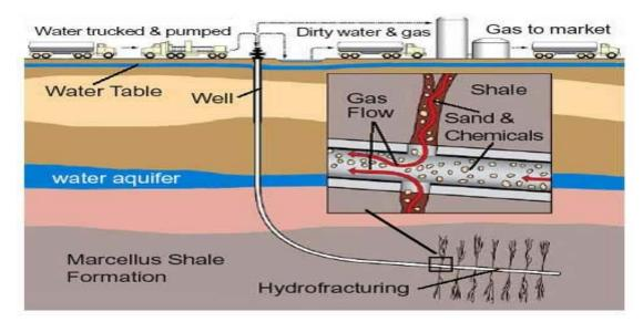
Figure 1.3 - Hydraulic fracturing process [5]
