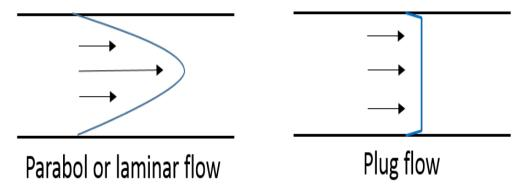
Figure 2.12 - Laminar flow in HPLC and plug flow in CE [51]
