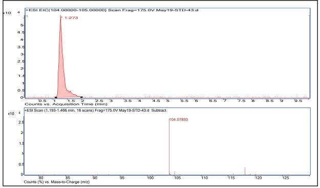
Figure C.2 - Extracted ion chromatogram and mass spectrum for choline ion present in sample 11243
