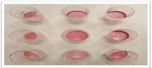
Figure 4.26 - Collected choline reinecke precipitates
