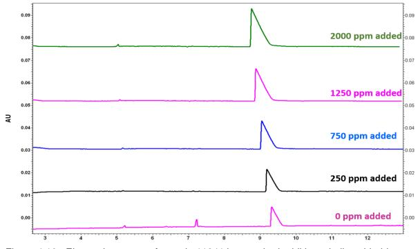
Figure 4.16 - Electropherogram of sample 11241 by standard addition; choline chloride spikes added (0 ppm, 250 ppm, 750 ppm, 1250 ppm, 2000 ppm)
