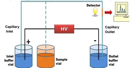
The light intensity *l<sub>in</sub>* through the capillary comes out with smaller intensity lout
