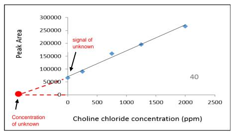
Figure 4.15 - Choline chloride concentration versus the peak area of choline ion based on standard addition method
