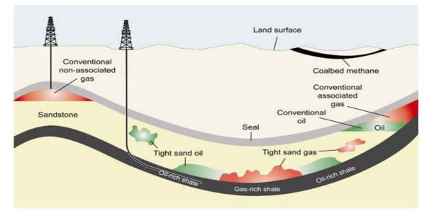
Figure 1.2 - Schematic geology of natural gas resources [3]
