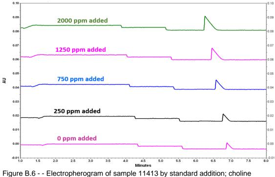
Figure B.6 - - Electropherogram of sample 11413 by standard addition; choline chloride spikes added (0 ppm, 250 ppm, 750 ppm, 1250 ppm, 2000 ppm)
