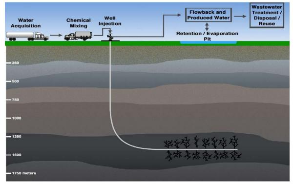
Figure 1.4 - Water management in oil and gas industry [8]
