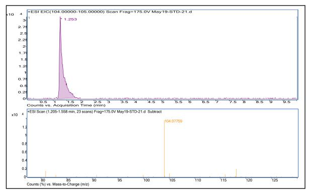
Figure C.5 - Extracted ion chromatogram and mass spectrum for choline ion present in sample 11411
