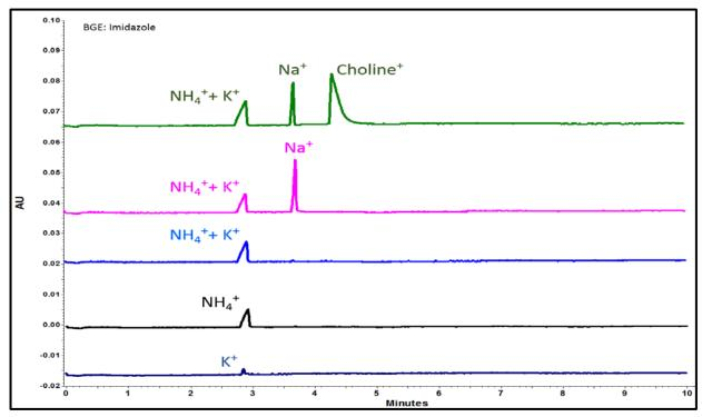
Figure 4.9 - Electropherograms of the separation of choline ion and ammonium, potassium, sodium ions by capillary electrophoresis with BGE containing imidazole
