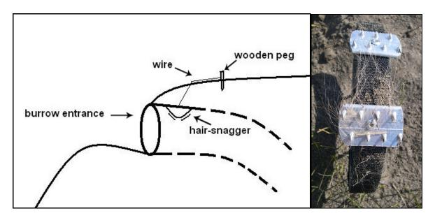
Figure 2.5. Schematic diagram (1) of hair-snagging device deployed in badger burrow and close up photo of hair-snagger (r) with suitable hair sample for DNA analysis. Each of the two snagging pinned knaplock segments were approximately 2.5 cm x 4 cm in dimension.
